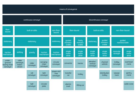
Figure 3 Classification of conveyor for transporting package goods according to Hompel (Hompel 2018 p.129)
